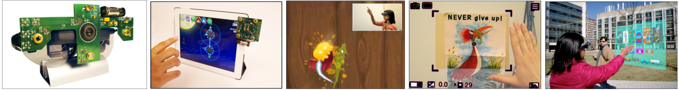
Figure 1. 3D Sensor Design and Interaction Scenarios: Mime is our compact, low power sensor for 3D gestural control of smart glasses. It comprises an active illumination three-pixel time-of-flight (TOF) sensor, and a 2D RGB camera. Mime's real-time signal processing pipeline enables fast and precise 3D gestural control in cluttered environments, and in strong daylight and dynamic light conditions.
